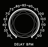
**DELAY BPM:** works as fine delay time adjustment, instead of milliseconds Beats Per Minute have been used as time measure unit.
